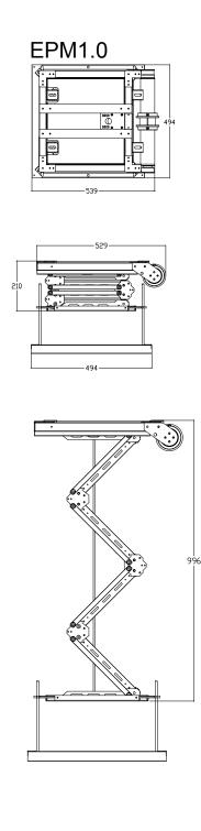
Ultra thin design, thickness is only 210mm, one-armed structure made from aluminum alloy, which can avoid the front- to-back and side-to-side swing problem. Arm sections: 4
