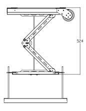
Ultra thin design, thickness is only 129mm, one-armed structure made from aluminum alloy, which can avoid the front- to-back and side-to-side swing problem. Arm sections: 2
