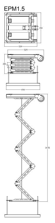
Ultra thin design, thickness is only 260mm, one-armed structure made from aluminum alloy, which can avoid the front- to-back and side-to-side swing problem. Arm sections: 6 Overall dimension: 453x528x281mm Ceiling opening: 500x500mm/550x550mm Traveling distance: 290–1500mm Distance from ceiling to false ceiling: 520–1500mm
